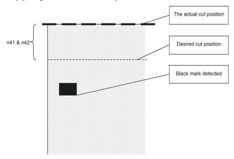
(ESC x n1 n2 is an obsolete command that sets n41 and n42. It is implemented for backward compatibility with old drivers. Set parameters n41 and n42 with the ESC & P n1 n2 command instead.)
